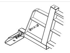
FASTEN EACH MOUNTING BRACKET TO THE HEAD RACK USING ONE 1/2"x3-1/4" HEX BOLT, TWO 1/2" FLAT WASHERS, ONE 1/2" LOCK WASHER AND ONE 1/2" HEX NUT
